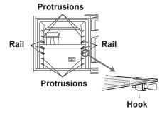
Do not remove the air inlet of the freezer compartment. If you remove them forcibly, it may cause deformation of the parts.
