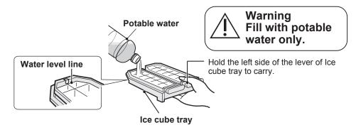
Do not overfill the tray with water. Otherwise the ice cubes will join together when frozen.
