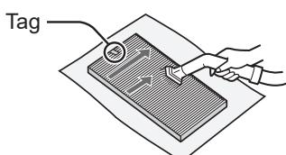
Gently remove dust from HEPA Filter and Deodorizing Filter with a vacuum cleaner attachment or similar tool.
