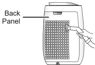
Gently remove dust from the back panel, using a vacuum cleaner attachment or similar tool.
