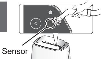
Gently remove dust from the sensor, using a vacuum cleaner attachment or similar tool.
