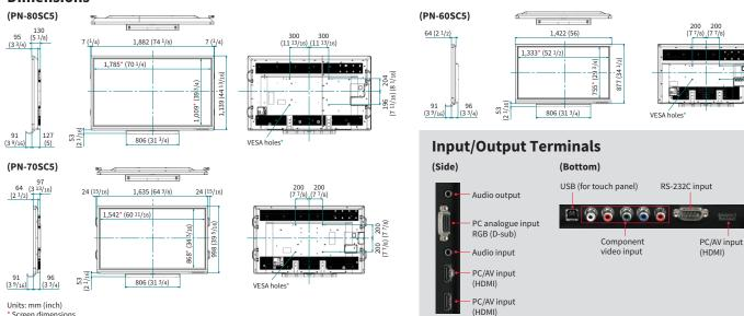
To use the VESA-standard mounting bracket, use M6 screws that are 8 to 10 mm plus the thickness of the bracket.
