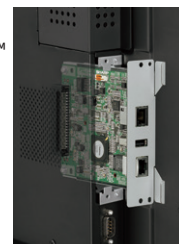
An optional board can slide into the slot on the back of the monitor.
