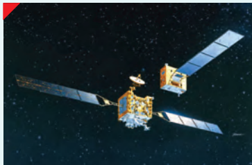
▲1976 The first Japanese operational Ionosphere Sounding Satellite "Ume" had 4,940 Sharp's photovoltaic modules on board for power supply.
